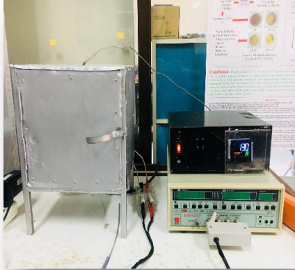
Dielectric Constant testing
