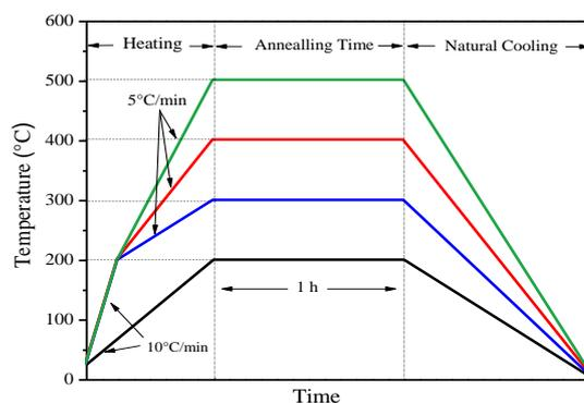
**Figure 3:** Schematic annealing temperature step of CZTS films
