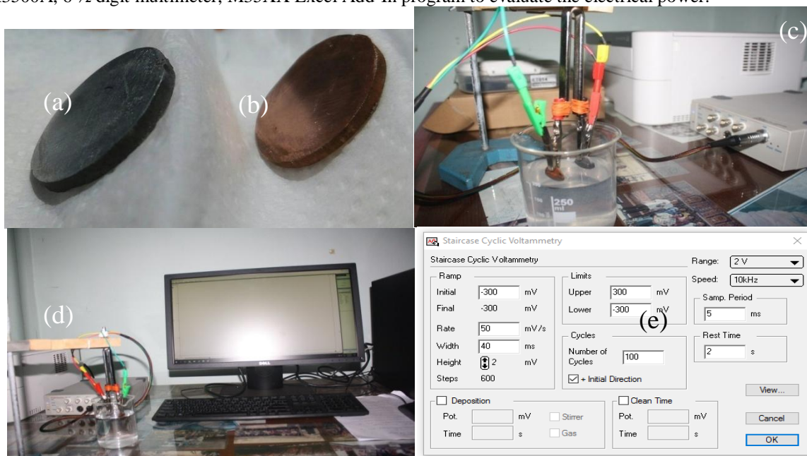
Figure 1: Cyclic voltammetry technique (a) Cu anode, (b) Al cathode, (c) dipping in NaCl+DI water, (d) connecting computer and (e) Staircase cyclic voltammetry
