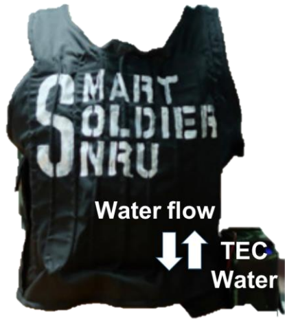
1 st TEC-water cooling
